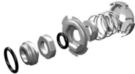
Fig. 6 Exploded view of shaft seal
